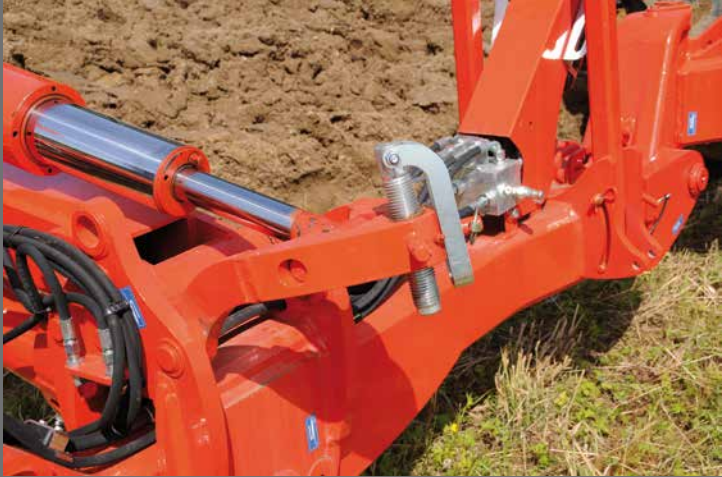
1. Levelling : by independent left / right crank screws for extra precision.
