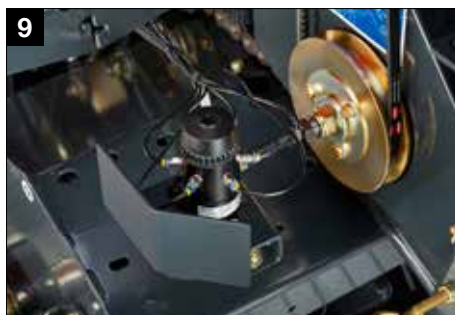
9 Beka Max continuous chain oiling system
